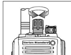
**Note:** Some models are programmed so that the operating channels are selected by the Programmable key and the memory channel group is selected by the **CH** selector knob. For further details, contact your VERTEX STANDARD dealer.
