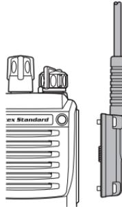
**!** *Note 1): Save the original plastic cap and its mounting screws. They should be reinstalled when not using the Speaker/Microphone.*
