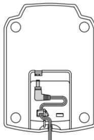
Insert the DC plug from the **PA-42** AC Adapter into the DC jack of the **CD-31** Desktop Rapid Charger.
