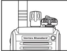
**MONITOR** button more than 2 seconds (or press the **MONITOR** button *twice*) to quiet the noise and resume normal (quiet) monitoring.
