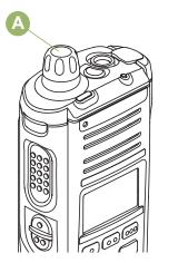
To increase the volume, rotate the **On/Off/Volume Control Knob** (<sup>(A)</sup>) clockwise.
