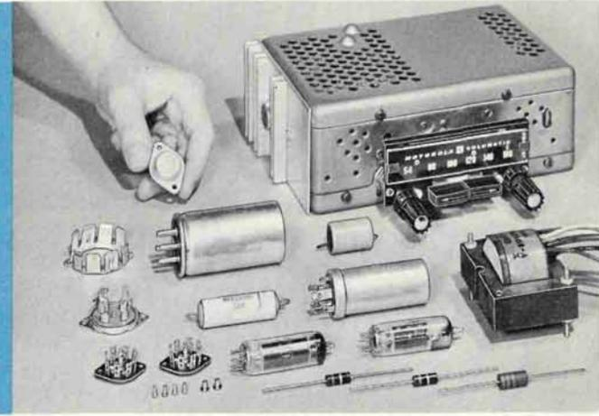
**New transistor powered car radios.** In some new Motorola car radios, this tiny transistor replaces all of the 20 parts shown next to it. In addition, transistors provide greater reliability and reduce battery drain.
