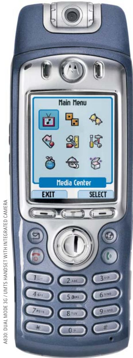
A830- DUAL MODE 3G / UMTS HANDSET WITH INTEGRATED CAMERA
