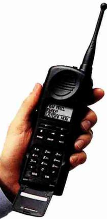
**The LINGO™ portable communicator is capable of accessing four wireless communications services: Voice Dispatch, Wireless Phone, Alpha Numeric Messaging and Data. It is used on networks based on the Motorola Integrated Radio System.**
