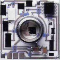
*Piezoresistive pressure sensors in electronic engine controls aid the precise control of air-fuel mixture.*
