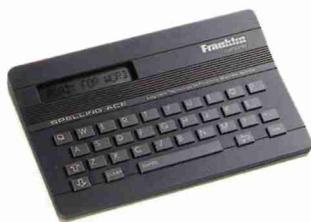
**A Motorola application specific IC controls liquid crystal display, logic and a memory of 80,000 words in this hand-held electronic speller from Franklin Computer Corp.**
