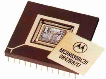
**The 32-bit MC68030 microprocessor provides twice the performance of first-generation 32-bit machines and maintains 100% upward software compatibility with the entire M68000 family.**
