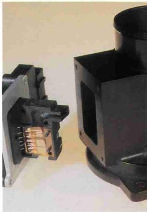
Mass air flow sensors, which directly measure the air mass inducted into an engine, are being field tested on customer vehicles.
