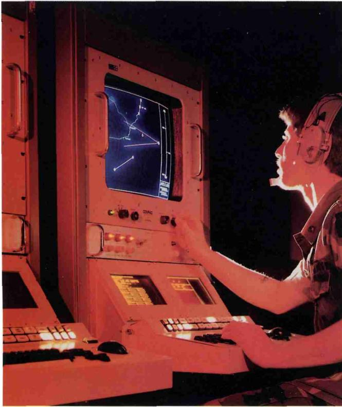
**This color raster scan display is part of the ground station module for Joint STARS, a joint-service radar-based surveillance system. GEG is the prime contractor for the ground station module, which is deployed with U.S. Army tactical operations centers and artillery command centers.**
