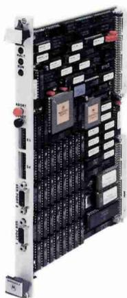
The MVME 140 multiprocessor board is the first such product to be based on Motorola's MC68030 second-generation 32-bit microprocessor.
