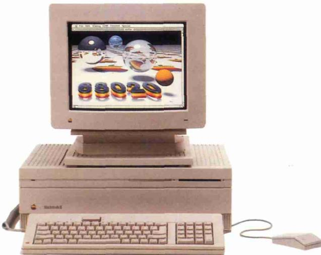
**Apple Computer's Macintosh II high-end personal computer is based on the 32-bit Motorola MC68020 microprocessor.**
