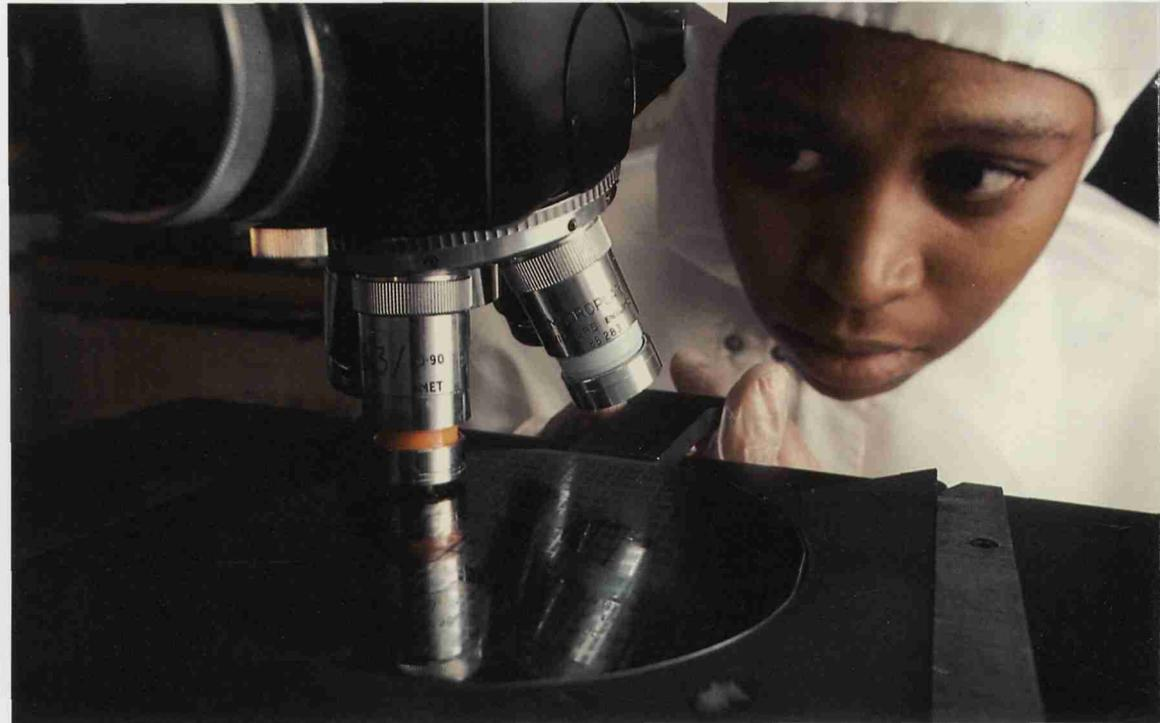
*(Above) As part of the photoresist process of wafer fabrication in the Mesa, Ariz., HMOS clean room, the critical dimensions of individual chips on the wafer are measured.*
