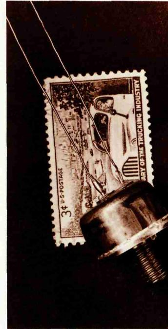
**1955** marked the formation of the then Semiconductor Division. One of the first products it manufactured was this germanium power transistor used in car radios.
