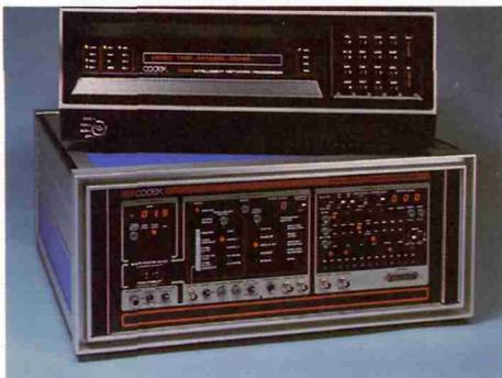
▲ Two of Codex's advanced data communications products, the 6030 Intelligent Network Processor and the Circuit Quality Monitoring System utilize Motorola 6800 microprocessor technology.
