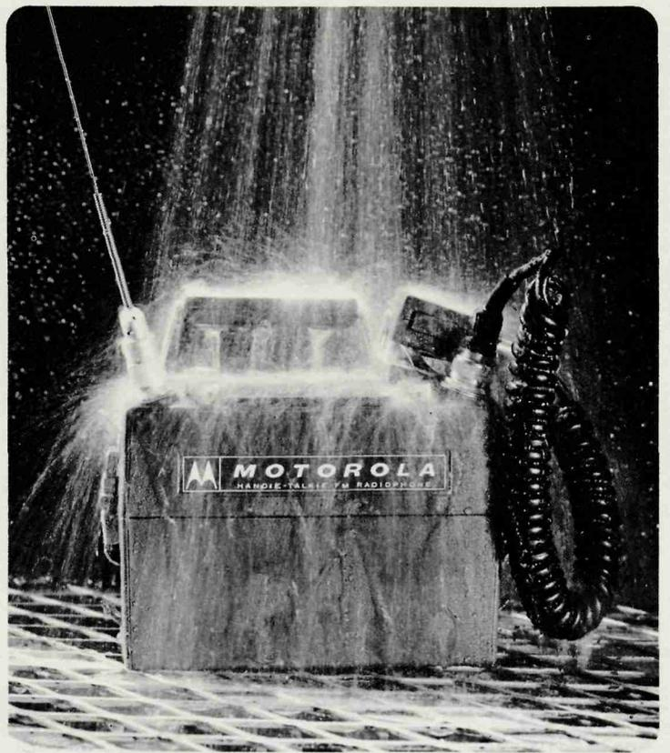
Lightweight 2-way portable radiophones, frequently used in inclement weather by such agencies as police departments, go through dust, cold and rain tests. Rigid standards of reliability are applied to all units.
