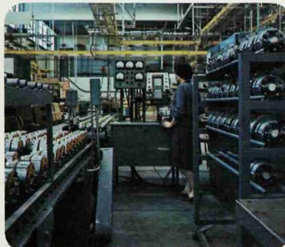
At this station in the Arcade facility, electronic alternators are given a series of electrical tests to check amperage, voltage, field current and noise levels.
