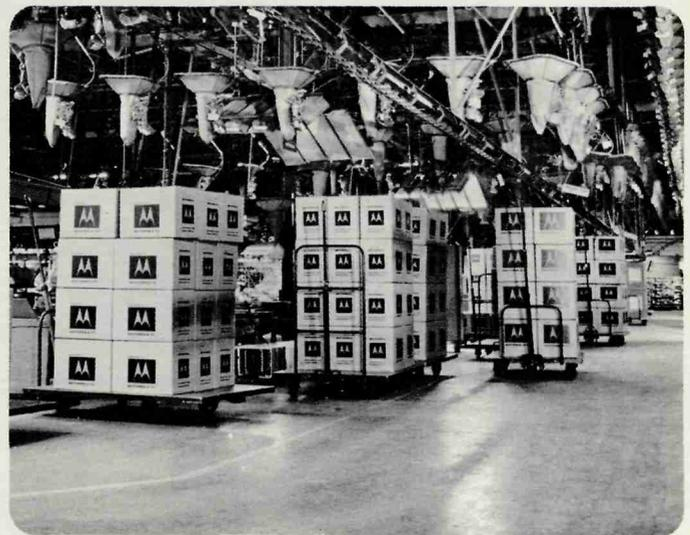
Conveyor systems add to efficiency in the production of black and white television sets. "Socks" hold picture tubes while hooks and platforms carry chassis to the lines for assembly. Corrugated boxes containing cabinets automatically roll along perimeter of manufacturing area to the proper stations for final assembly.
