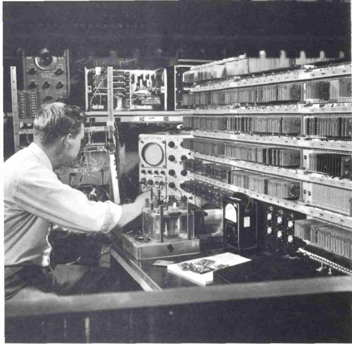
Airborne digital computers undergoing reliability tests above are examples of the "sophisticated hardware" being developed by technical personnel in Motorola's Military Electronics Division.
