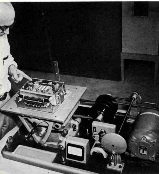
▲ **Shaking out the "bugs."** One way Motorola works to stop trouble before it starts is shown by this vibration table at the Quincy car radio plant. Units from the assembly lines are placed on this table and subjected to vibrations and stresses far more severe than any they will get in actual use. Thus potential difficulties are discovered and nipped in the bud.
