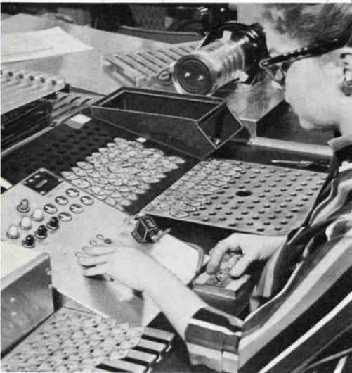
▲ **Transistorized sleuthing.** In-process manufacturing tests at the Phoenix, Arizona, transistor plant are made with special jigs designed and built by Motorola. Used to check the many electrical characteristics of transistors, these jigs are themselves fully transistorized.
