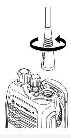
Turn the antenna counterclockwise to remove it.
