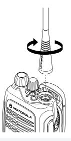
Turn the antenna clockwise to attach it.
